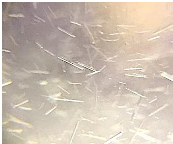
Figure 4.9. Self-assembly of macrocycle 1 results in the formation of needle-like crystals upon recrystallization in DMSO. Picture taken at 60x magnification with a LED pocket microscope.
